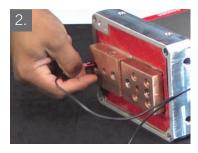
First, connect the CTF positive lead to the MFDC negative pad, as shown in figure 2.
