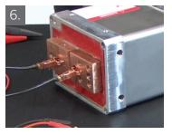
First, be sure to protect the MFDC diodes by connecting the jumper wires one end to each of the two MFDC pads, as shown in figure 6.
