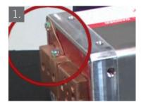
Be sure to remove the ground strap, as shown in figure 1, before any testing. The test results will not be accurate if the ground strap is left on. Also, be sure to clean off any weld flash and debris from the secondary pads and primary connections.
